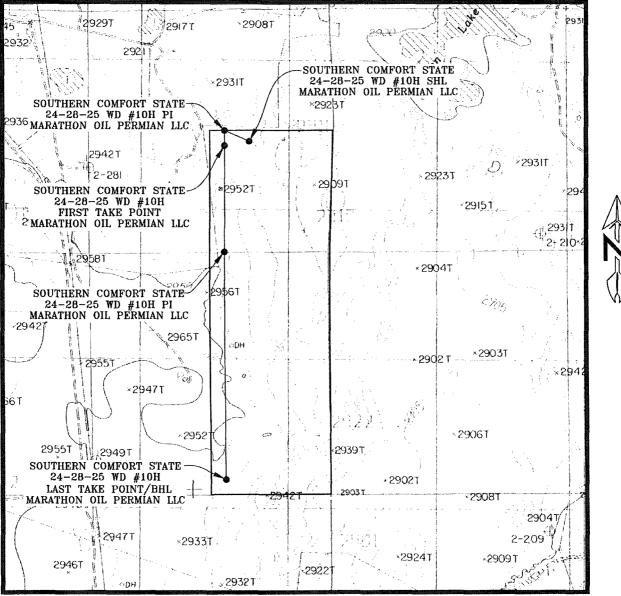
SEC. 24 TWP. 24-S RGE. 28-E SURVEY: N.M.P.M. COUNTY: EDDY DESCRIPTION: 2424' FSL & 1838' FEL ELEVATION: 2918' OPERATOR: MARATHON OIL PERMIAN LLC LEASE: SOUTHERN COMFORT STATE 24-28-25 U.S.G.S. TOPOGRAPHIC MAP: MALAGA, N.M. SCALE: 1" = 2000' CONTOUR INTERVAL = 10'
