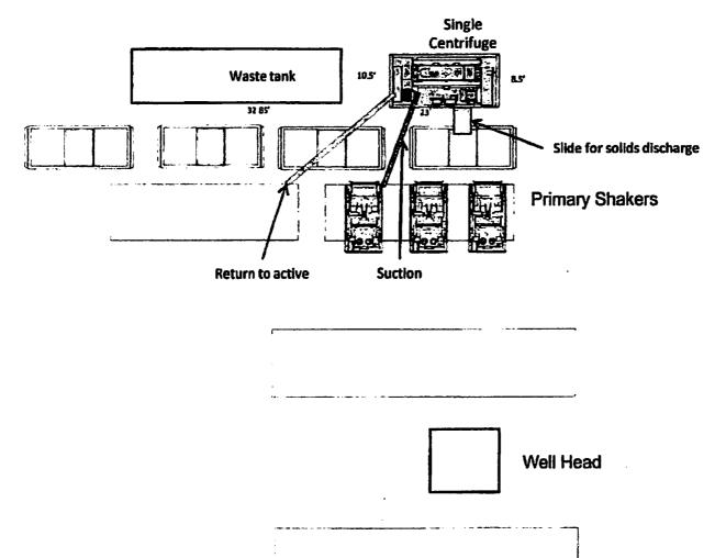
Oxy Single Centrifuge Closed Loop System – New Mexico Flex III May 28, 2013
