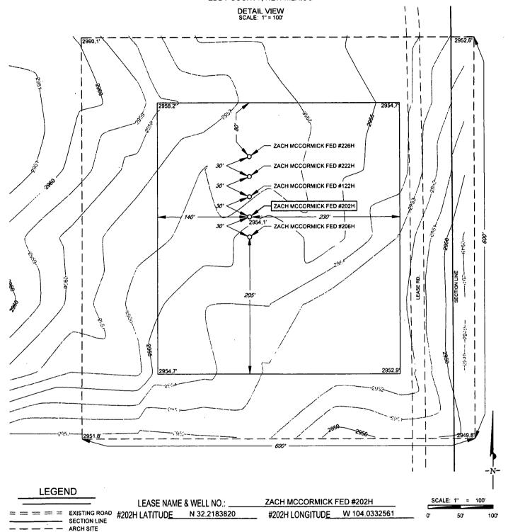
ALL BEARINGS, DISTANCES, AND COORDINATE VALUES CONTAINED HEREON ARE GRID BASED UPON THE NEW MEXICO STATE PLANE COORDINATE SYSTEM, EAST ZONE OF THE NORTH AMERICAN DATUM 1983, U.S. SURVEY FEET
