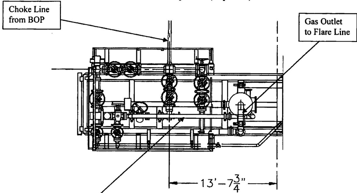
**Choke Manifold – Gas Separator (Side View)**
