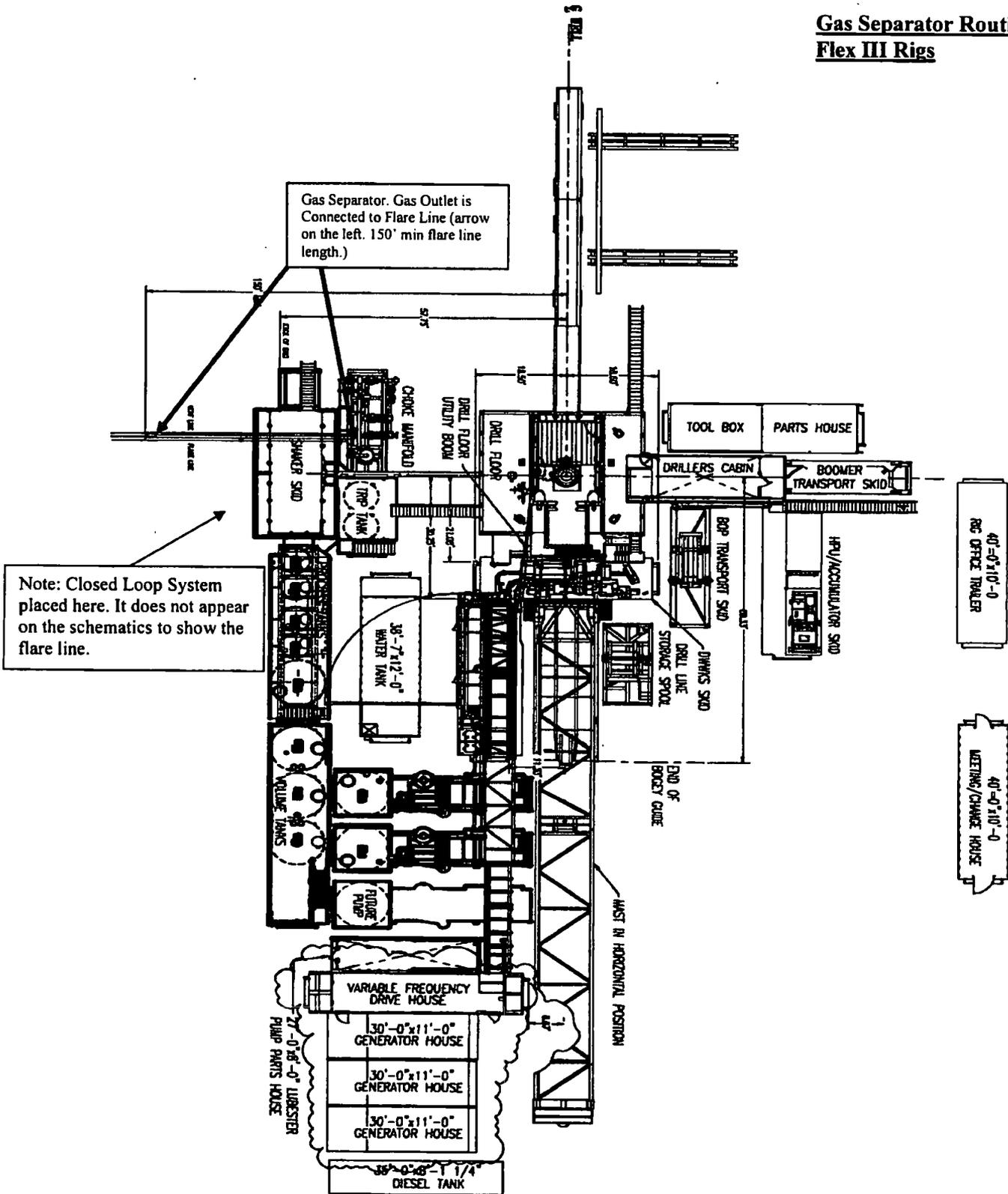
**Choke Manifold – Gas Separator (Top View)**
