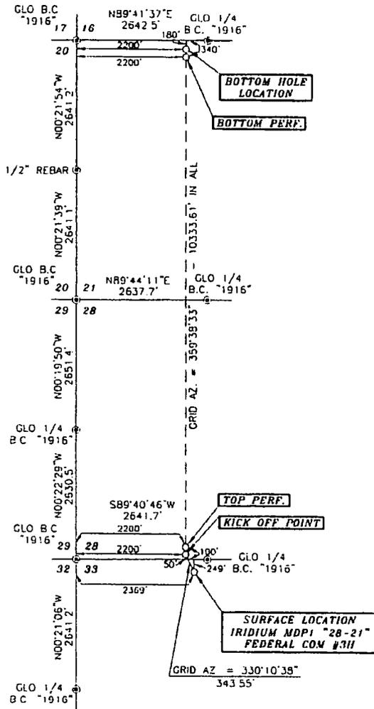
Basis of Bearings - CPS Geosidic Measurements
