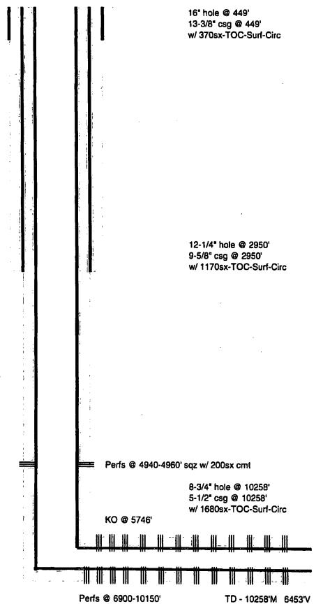
TD - 10258'M 6453'V PB - 10198'M 6454'V OXY USA Inc. - Proposed Cedar Canyon 28 Federal Com. #2H API No. 30-015-41073
