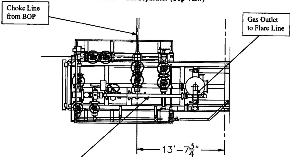
**Choke Manifold – Gas Separator (Side View)**
