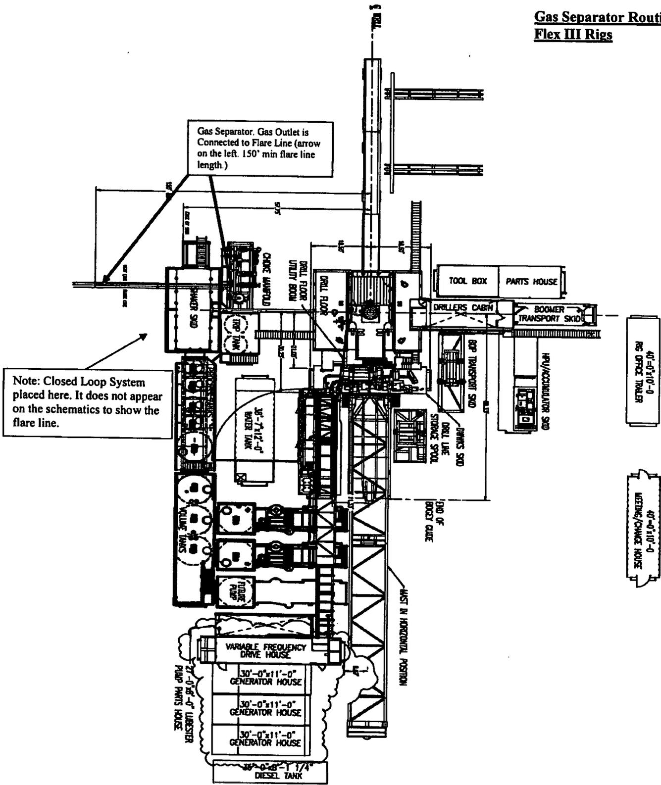
**Choke Manifold – Gas Separator (Top View)**
