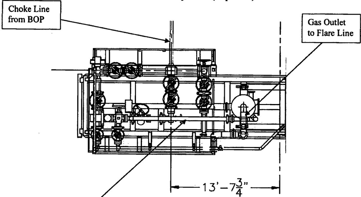
**Choke Manifold – Gas Separator (Side View)**
