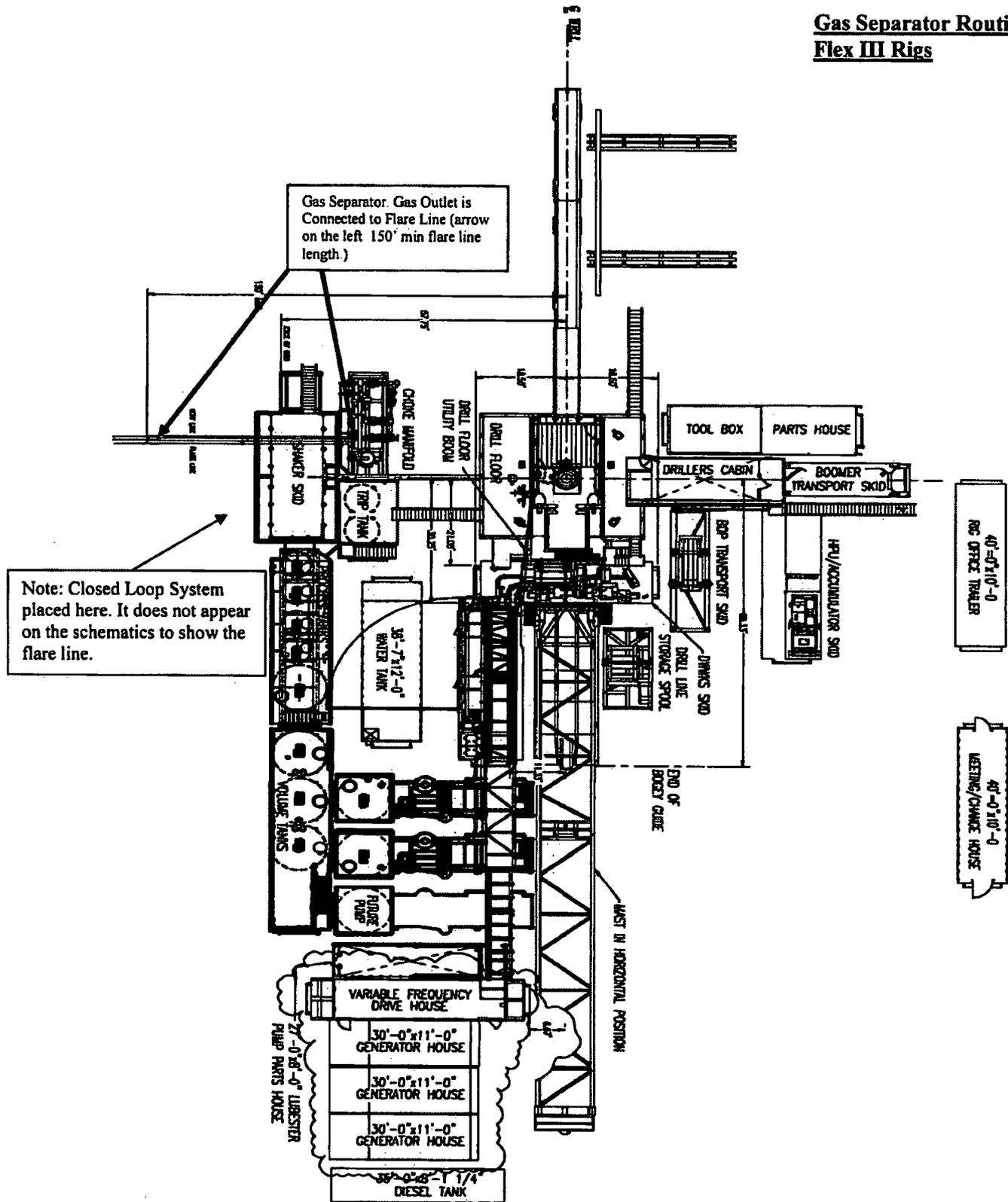
**Choke Manifold – Gas Separator (Top View)**
