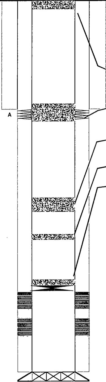
Spot a 10 SX (95 ft) CLS C cement plug 0 ft - 95 ft. WOC & Tag Plug. This will plug the Top and cover hole in casing.
