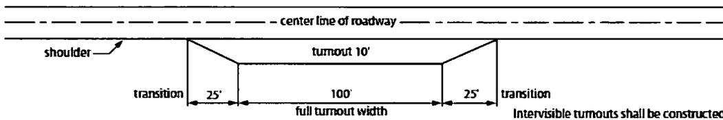
Intervisible turnouts shall be constructed on all single lane roads on all blind curves with additional turnouts as needed to keep spacing below 1000 feet.
