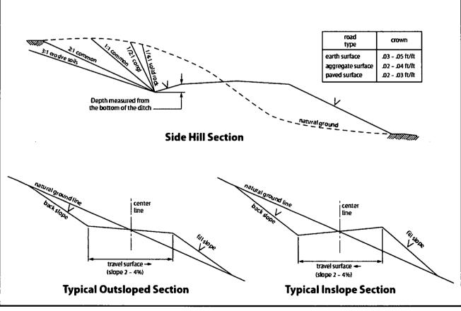
Figure 1. Cross-sections and plans for typical road sections representative of BLM resource or FS local and higher-class roads
