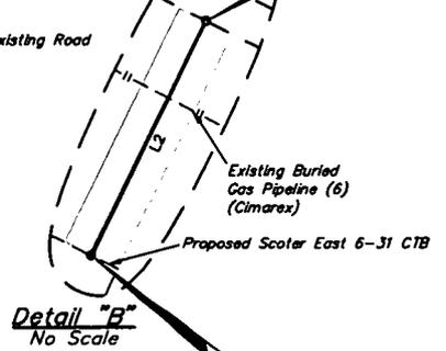
END OF PROPOSED ROAD "B" RIGHT-OF-WAY (At Edge of Proposed Scooter East 6-31 Federal COM CTB)
