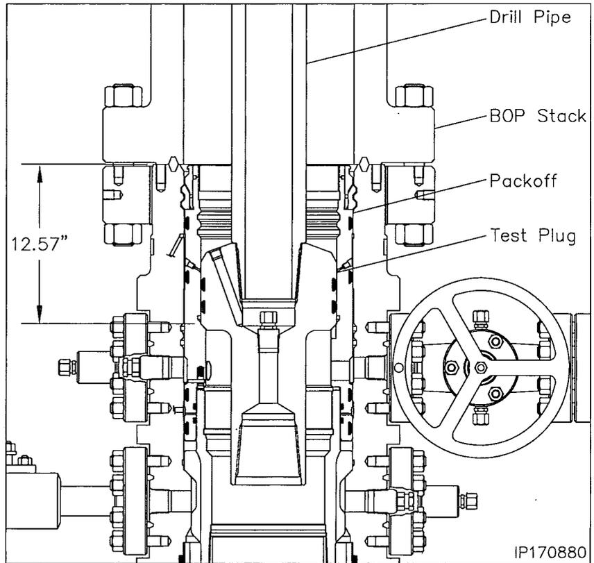
9. Remove as much fluid as possible from the BOP stack and the retrieve the test plug with a straight vertical lift.
