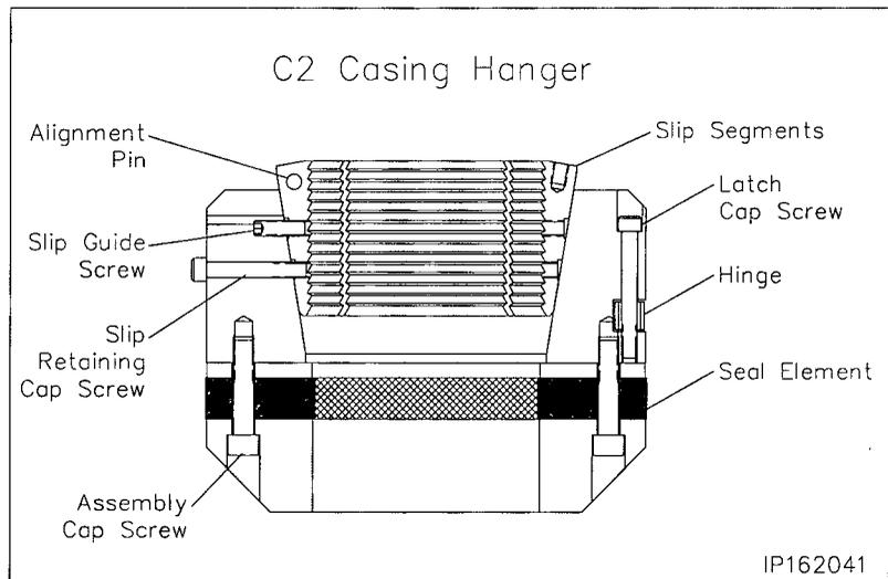
**Note:** Side outlet valve to remain open while setting the casing hanger.
