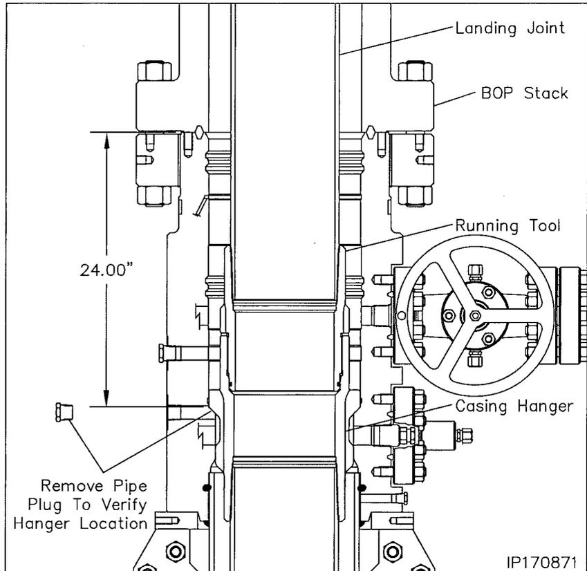
26. **Using Chain Tongs Only located 180° apart,** retrieve the Running Tool and landing joint by rotating the landing joint clockwise (right) approximately 16 turns.
