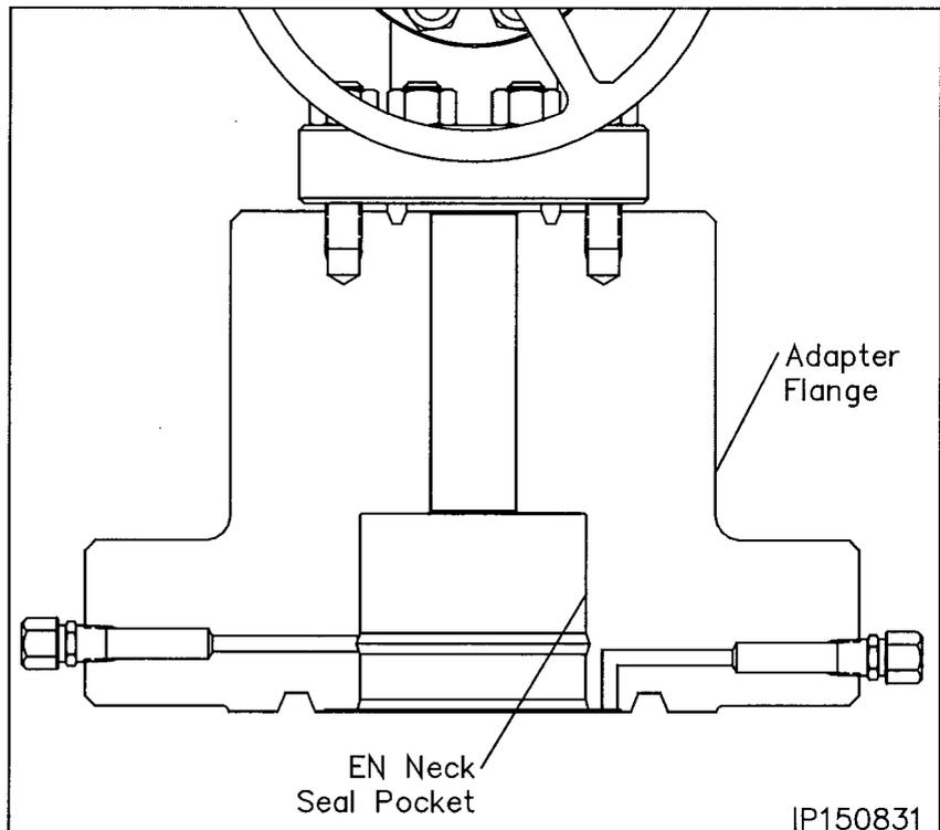
7. Lightly lubricate the adapter seal pocket and ring groove with oil or a light grease.
