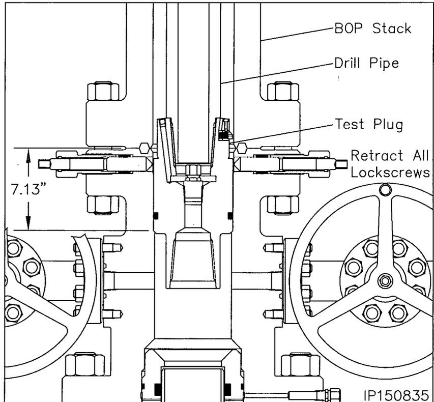
6. Carefully lower the test plug through the BOP and land it on the load shoulder in the tubing head, 7.13" below the top of the head.
