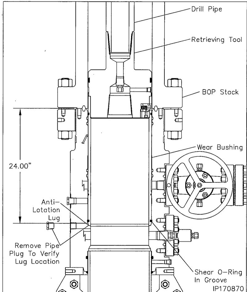
**Note:** The Shear O-Ring on bottom of the bushing will locate in a groove above the load shoulder in the head to act as a retaining device for the bushing.
