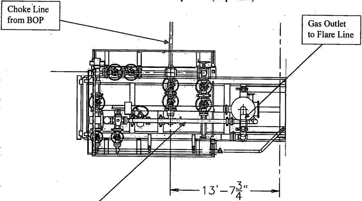
**Choke Manifold – Gas Separator (Side View)**
