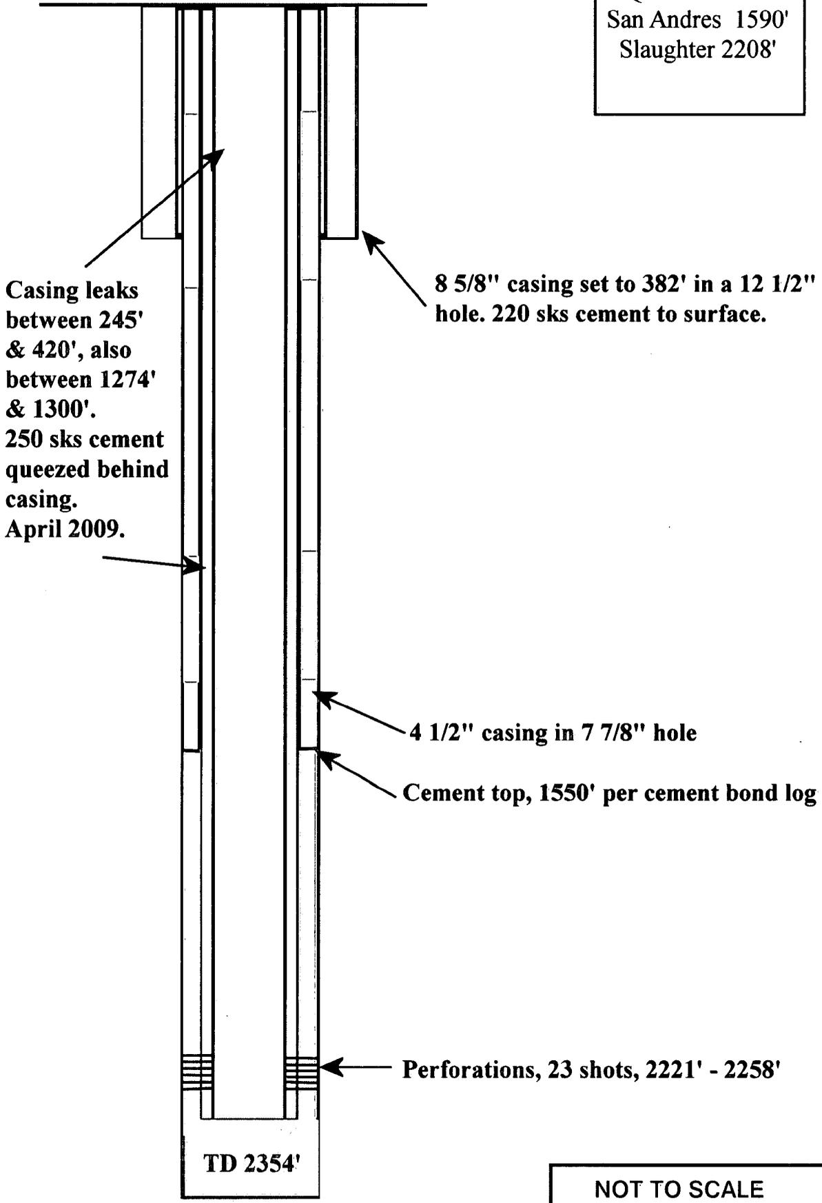
Casing leaks between 245' & 420', also between 1274' & 1300'. 250 sks cement queezed behind casing. April 2009.
