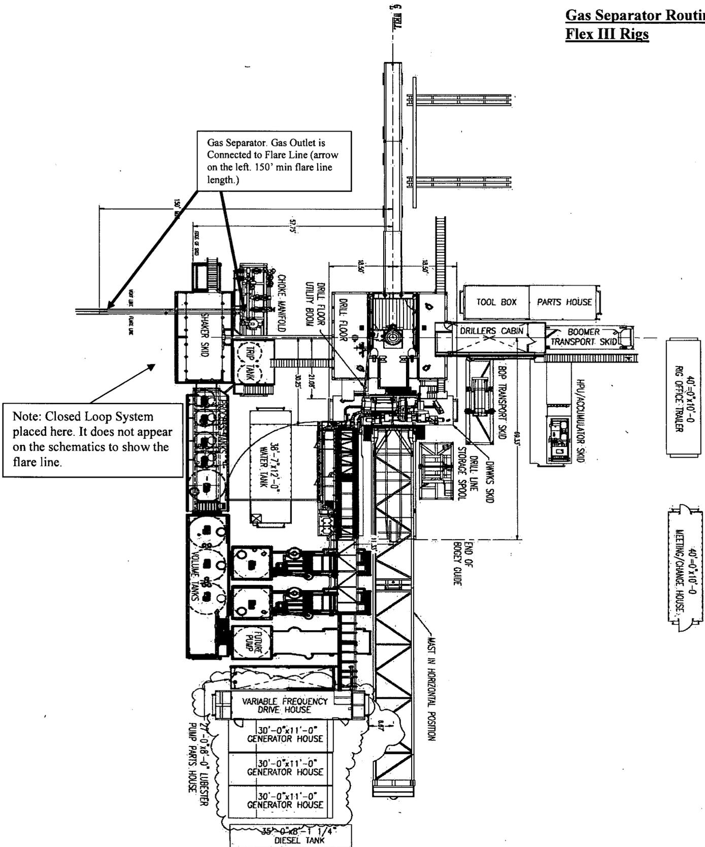
**Choke Manifold – Gas Separator (Top View)**
