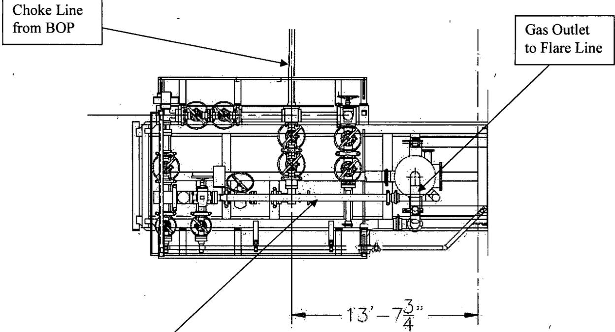
**Choke Manifold – Gas Separator (Side View)**
