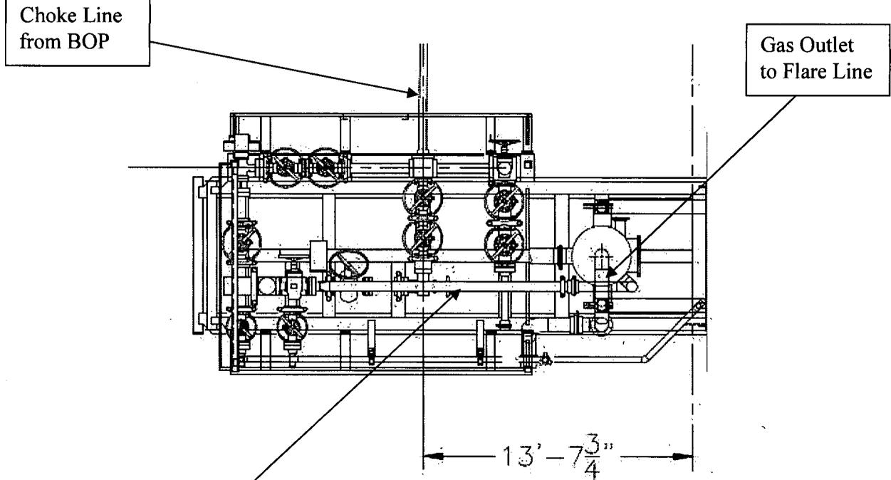
**Choke Manifold – Gas Separator (Side View)**
