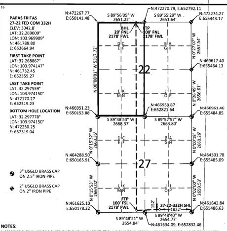
1. BEARINGS SHOWN ARE GRID BASED ON THE NEW MEXICO STATE PLANE EAST ZONE COORDINATE SYSTEM (3001), NAD 83 (2011), BASED FROM GPS OBSERVATIONS, OCCUPYING A WHS CONTROL POINT (5/8" REBAR), LOCATED AT NORTH: 456034.443, EAST: 653560.6 41, ELEVATION: 3101.373, DETERMINED BY AN OPUS SOLUTION ON DECEMBER 3RD, 2018.
