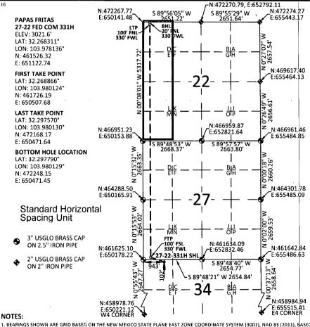
1. BEARINGS SHOWN ARE GRID BASED ON THE NEW MEXICO STATE PLANE EAST ZONE COORDINATE SYSTEM (3001), NAD 83 (2011), BASED FROM GPS OBSERVATIONS, OCCUPYING A WHS CONTROL POINT (5/8" REBAR), LOCATED AT NORTH: 456034.443, EAST: 653560.641, ELEVATION: 3101.373, DETERMINED BY AN OPUS SOLUTION ON DECEMBER 3RD, 2018.
