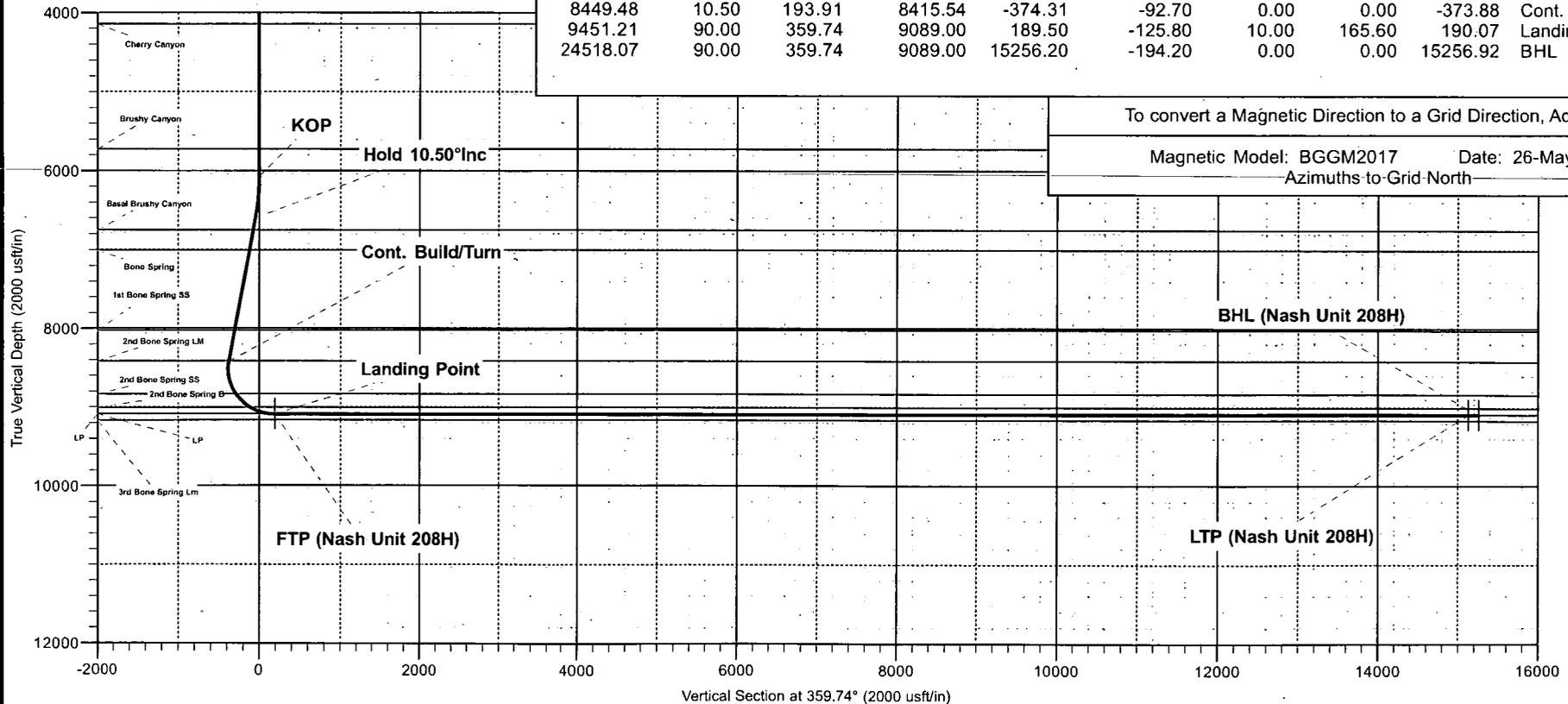
To convert a Magnetic Direction to a Grid Direction, Add 6.98°
