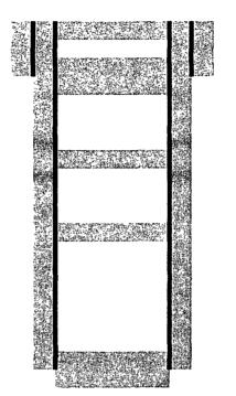
17-1/2" hole @ 694' 13-3/8" csg @ 694' w/715sx-TOC-Surf-Circ
