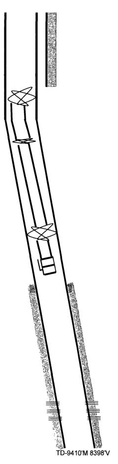
12-1/4" hole @ 1620' 9-5/8" csg @ 1620' w/1130sx-TOC-Surf-Circ
