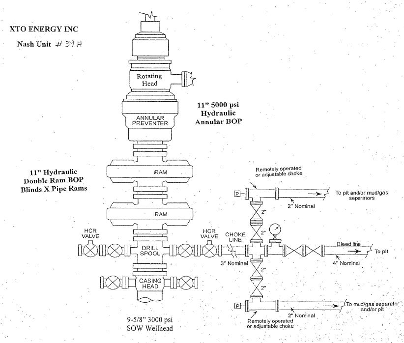
5000 psi Working Pressure BOPE Configuration and Choke Manifold
