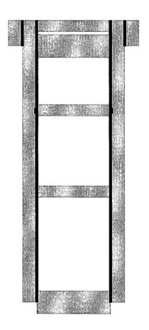
17-1/2" hole @ 340' 13-3/8" csg @ 340' w/400sx-TOC-Surf-Circ
