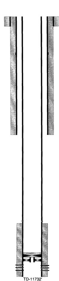
17-1/2" hole @ 340' 13-3/8" csg @ 340' w/400sx-TOC-Surf-Circ
