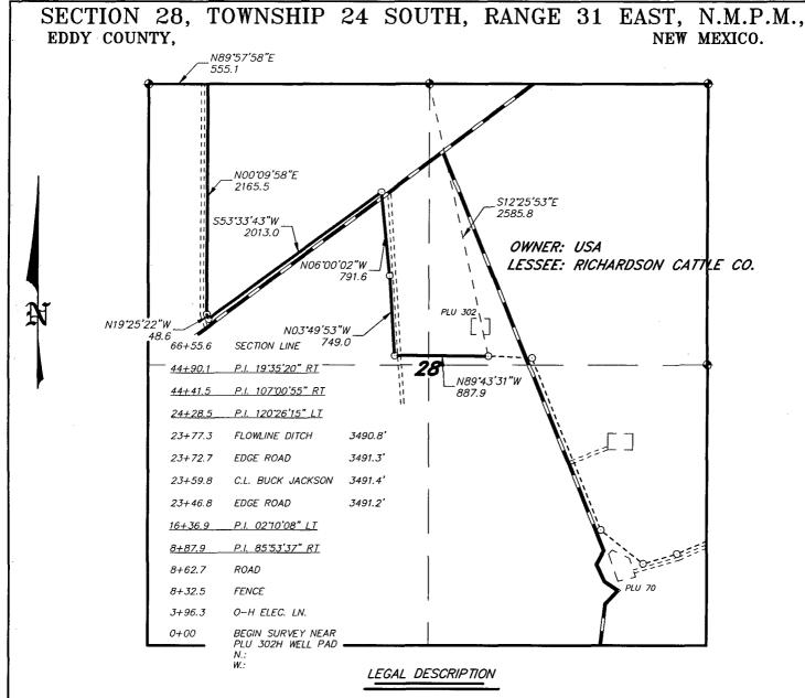
A STRIP OF LAND 30.0 FEET WIDE, LOCATED IN SECTION 28, TOWNSHIP 24 SOUTH, RANGE 31 EAST, N.M.P.M., EDDY COUNTY, NEW MEXICO AND BEING 15.0 FEET LEFT AND RIGHT OF THE ABOVE PLATTED CENTERLINE SURVEY.
