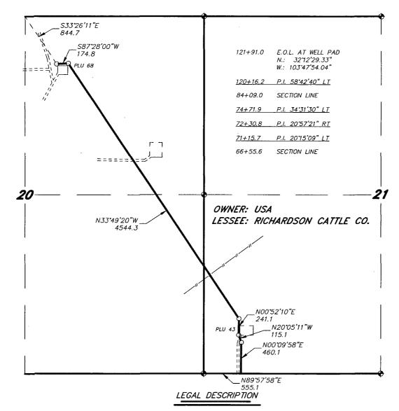
A STRIP OF LAND 30.0 FEET WIDE, LOCATED IN SECTION 20&21 TOWNSHIP 24 SOUTH, RANGE 31 EAST, N.M.P.M., EDDY COUNTY, NEW MEXICO AND BEING 15.0 FEET LEFT AND RIGHT OF THE ABOVE PLATTED CENTERLINE SURVEY.
