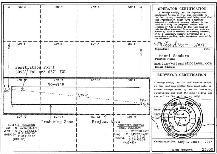
Units: Feet, °, 7100ft Tgt TVD: 7310.00 Co: 0 VS Az: 95.83 Drillers: 0 Elevation: Tgt Radius: 0.00 Tgt MD: 0.00 Well Name: Grande Mike AZK State 3H Northing: Tgt N/S: -486.60 Tgt Displ.: 0.00 Location: Sect. 2, 16S-29E Tgt E/W: 4768.86 Method: Minimum Curvature Easting:
