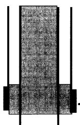
Perforate casing 50' above 8 5/8" casing shoe and circulate cement to surface in and out.
