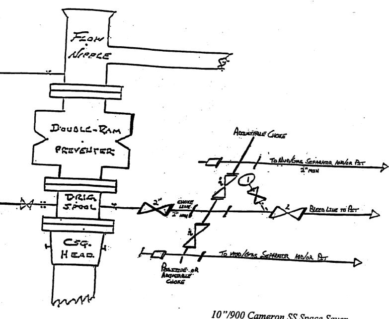
Marbob Energy Corporation Muskegon South State No. 1 1650' FSL & 330'FEL Section 20; T17s – R29e Eddy County, New Mexico 10"/900 Cameron SS Space Saver 3000# Working Pressure 3000# Working Pressure Choke Manifold DISTRICT I P.O. Bez 1980, Hobbs, NM 88241-1980
