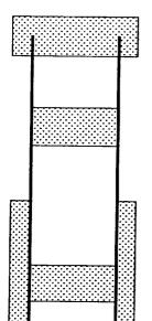
50 SX CEMENT PLUG: 854'- 1084' (TOP OF SALT @ 960') CUT OFF 5 1/2" CASING @ 1035'
