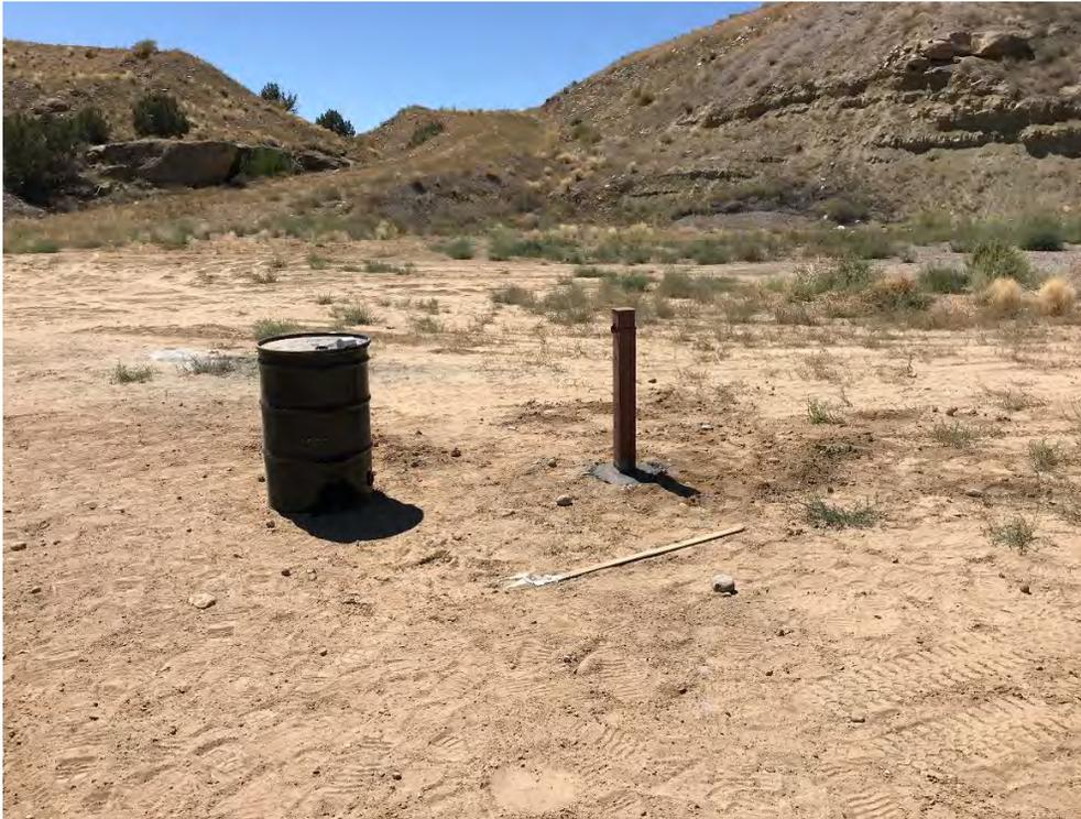
**Photograph 8:** MW03 completed well, 35 feet.
