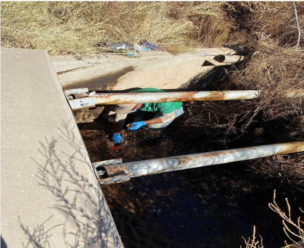
Photograph 8. Collecting surface soil sample SS-8 at southern culvert.
