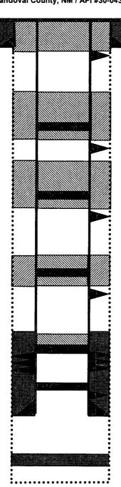
9-5/8" Casing set @ 100' Cement with 100 sxs (Circulated to Surface)
