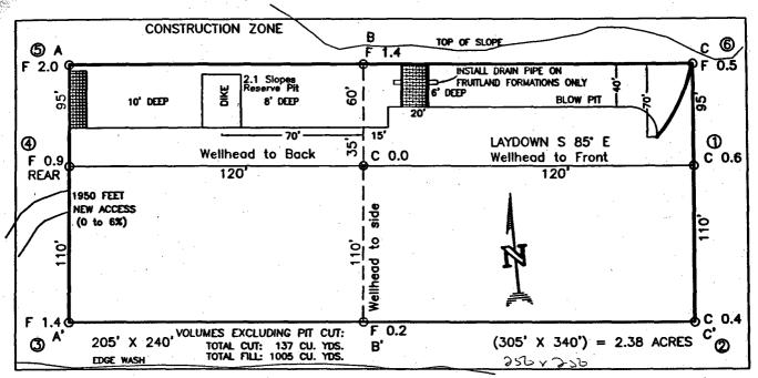
RESERVE PIT DIKE: TO BE 8' ABOVE DEEP SIDE (OVERFLOW - 3' WIDE AND 1' ABOVE SHALLOW SIDE). BLOW PIT: OVERFLOW PIPE HALFWAY BETWEEN TOP AND BOTTOM AND TO EXTEND OVER PLASTIC LINER AND INTO BLOW PIT.
