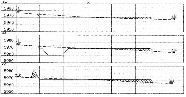
stakes are approximate and include additional areas r for sideslopes and drain Final Pad Dimensions of
