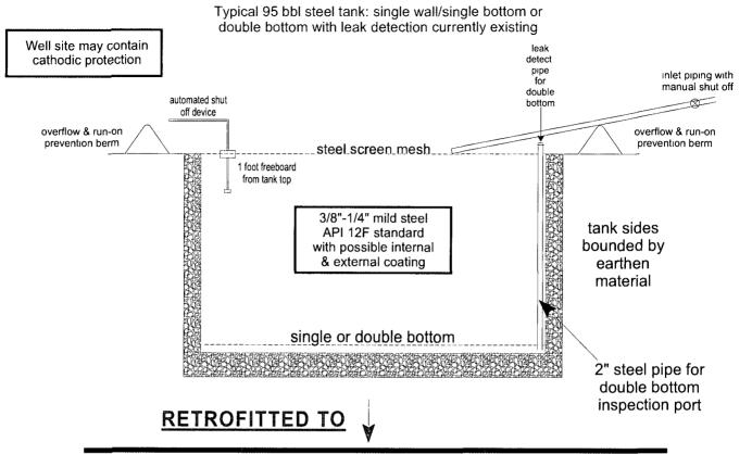
21/45/50 bbl steel tank: single wall / single bottom or double bottom with leak detection inserted into 95 bbl steel tank: single wall / single bottom or double bottom with leak detection / 6" lift
