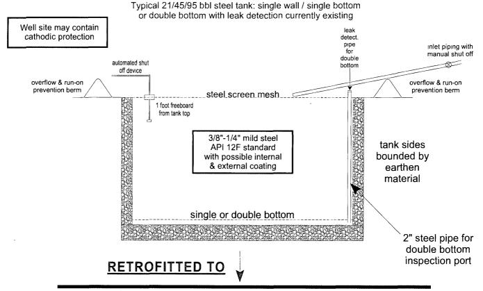
21/45/95 bbl steel tank: single wall / single bottom or double bottom with leak detection / visible sides / 6" lift / geomembrane liner
