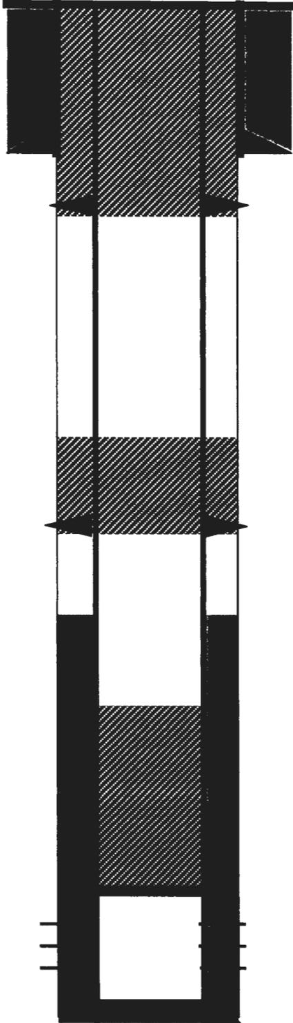
7-5/8" 26.4# casing @ 120'. Cemented with 50 sks Cement. Hole size 9-3/4"
