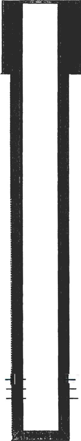
7", 20# casing @ 103'. Circulated cement to surface.
