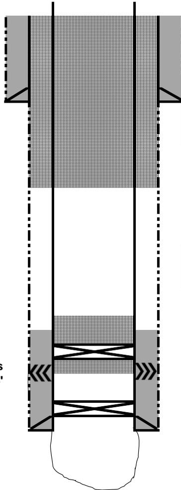
**Plug 2:** Perforate 4 holes 50' below top of Fruitland. Tie on to 5-1/2" casing, and mix and pump sufficient Class G cement to bring to surface inside and outside 5-1/2" casing.
