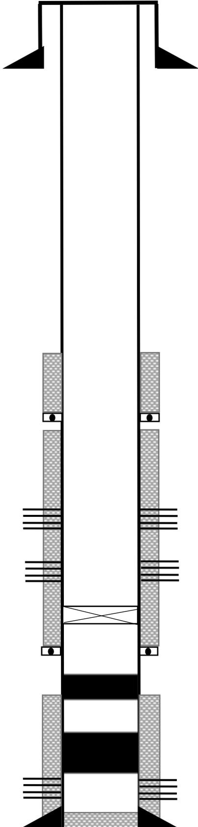
8-5/8", 24# casing @ 236'. Cemented to surface.
