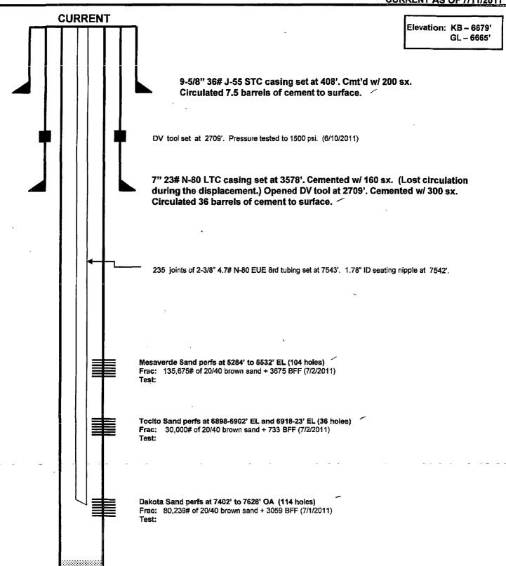
TD: 7675' PBTD: 7624' 4-1/2" 11.6# N-80 LTC casing set at 7665'. (Marker joint at 4966'.) Cmt'd w/ 220 sx. Estimated top of cement at 3550' (CBL). ✓
