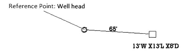
From Reference Point Go S 60 Degrees SE.For a Distance of 65' to Center of pit.
