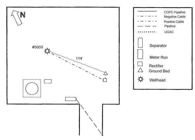
Drill ground bed approximately 114' south east of #500S wellhead at staked location. Install single well solar unit, and install cables to new ground bed and #500S wellhead at lengths below.
