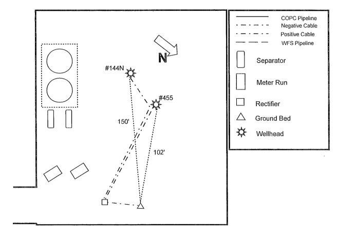
Drill ground bed approximately 102' East of #455 wellhead at staked location. Install three well solar unit, and install cables to new ground bed and #144N and #455 wellheads at lengths below.
