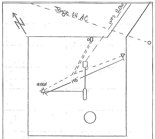
Drill ground bed 198' East of wellhead at staked location. Install Weter Pole and 40-16 3 neg., install coblex to new ground bed and #100 wellhead at lengths listed below.
