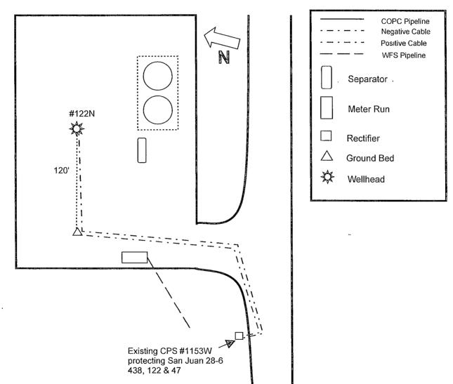
Drill ground bed approximately 120' west of #122N wellhead at staked location. Upgrade existing CPS #1153W to 60-30 rectifier, install cables to new ground bed, #122N wellhead at lengths below, and reconnect any existing ground bed positive cables and wellhead negative cables for the following wells: San Juan 28-6 Unit 438, 122 & 47.
