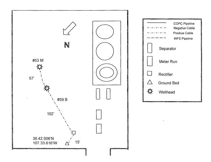
Drill ground bed approximately 108' south west of #59 B well head at staked location. Install solar rectifier at staked location. Install cable to new ground bed and to #59 B and #53 M wellhead's at lengths below.
