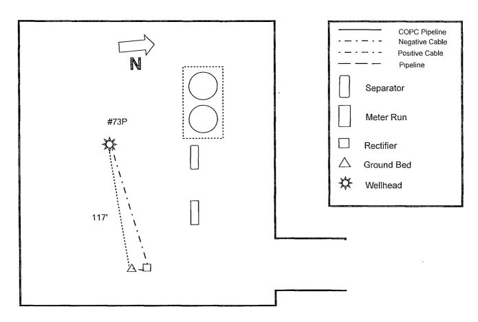
Drill ground bed approximately 117' East of #73P wellhead at staked location. Install single well solar unit, and install cables to new ground bed and #73P wellhead at lengths below.
