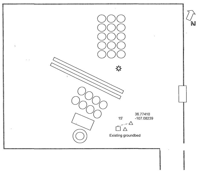
Drill ground bed at staked location approximately 15'northeast of rectifier and load w/15 anodes. Connect positive cable to existing rectifier.
