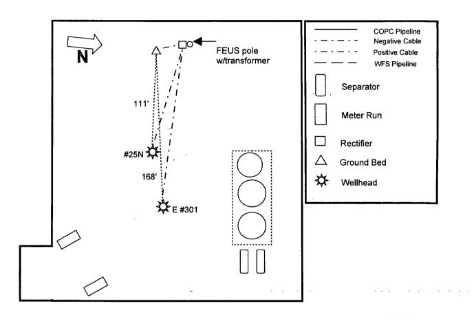
Drill ground bed approximately 111' west of #25N wellhead at staked location. Install 40-16 3 Negative rectifier on FEUS pole, and install cables to new ground bed and #25N and Howell E #301 wellheads at lengths below.
