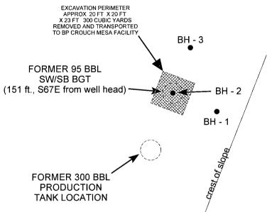
BORING LOGS & BELOW-GRADE TANK LOCATIONS ARE ONLY AS ACCURATE AS THE INSTRUMENTS USED IN OBTAINING THE FOOTAGE & BEARING FROM THE WELL HEAD (TAPE MEASURE, LASER RANGE FINDER, & BRUNTON COMPASS). ALL OTHER STRUCTURES DISPLAYED ON THIS MAP ARE SOLELY FOR REFERENCE AND MAY NOT BE TO SCALE MAGNETIC DECLINATION USED ~ 10° E
