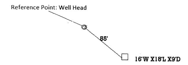
From Reference Point Go N.35 Degrees NE. For a Distance of 85' to Center of Pit.
